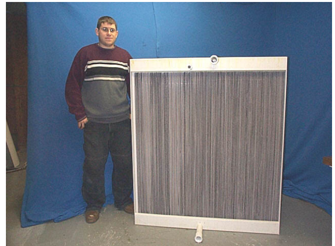
Figure 3 – 6,000 cfm Low-Flow Liquid-Desiccant Conditioner
