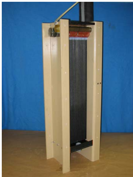
Figure 5 – A Low-Flow Scavenging-Air Regenerator
