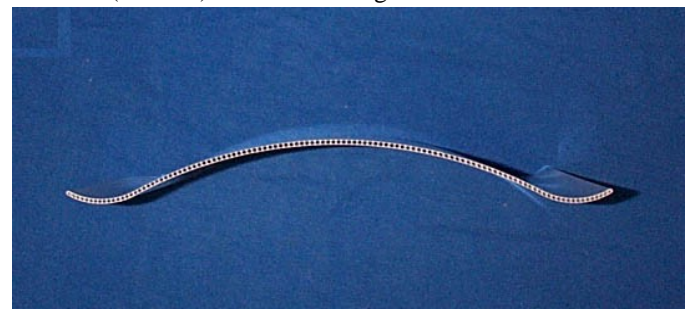
Figure 4 – Cross Section of Plate Extrusion
